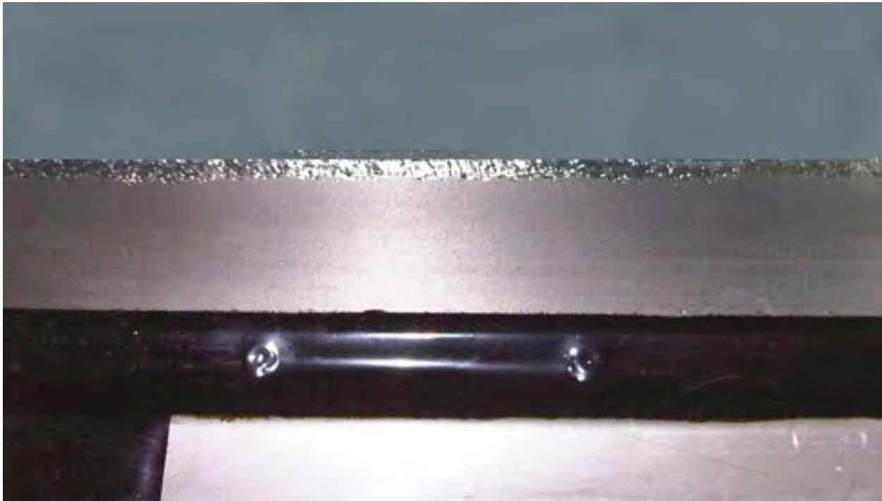
The edges of the panel have been ground to present as small a transition as possible.
