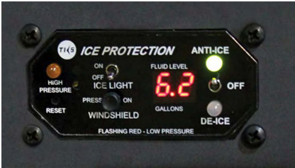
TKS Ice Protection System Control Panel.
