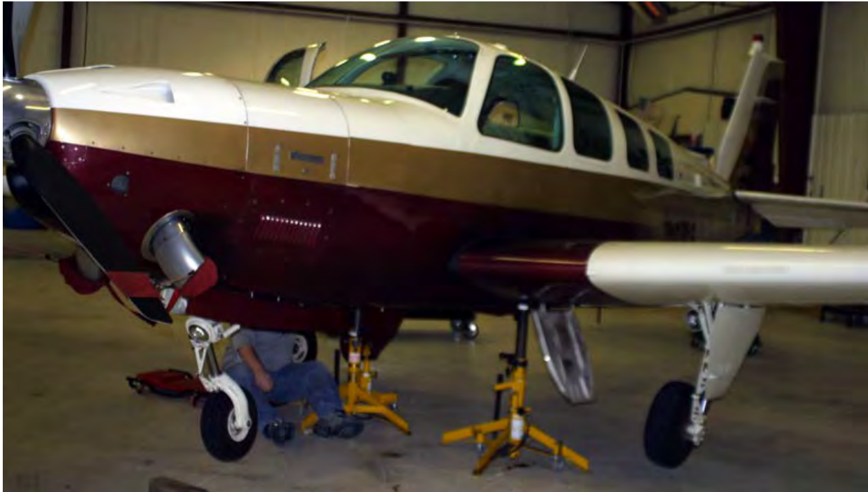
The plane is first put on jacks. Gear doors need to be lowered for the installation. The pump, filter, windshield pump, solenoid and pressure switches will be installed in the right wheel well.
