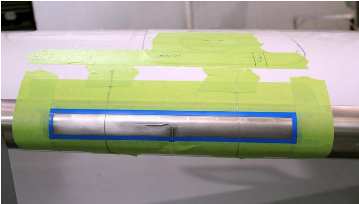
Locations where the stall strips will be installed are taped and prepared. The stall strips are filled with a foam material that spreads the fluid along the entire surface.
