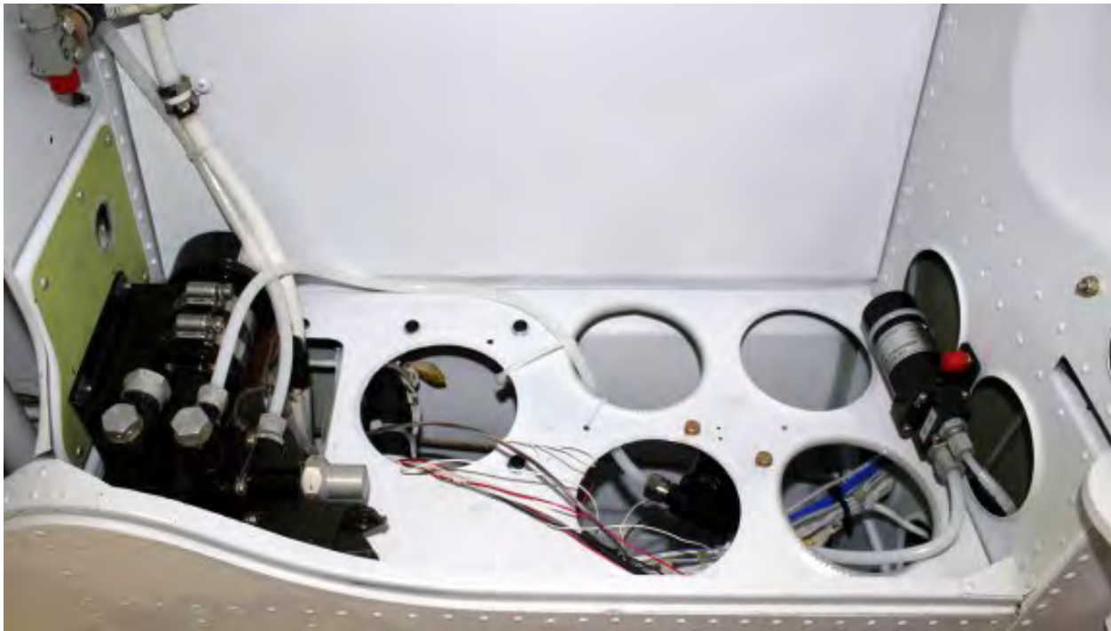
The main pump and windshield pump are also located in the wheel well (aft view). Hidden from view, the solenoid's position is evident if you follow the tubing.
