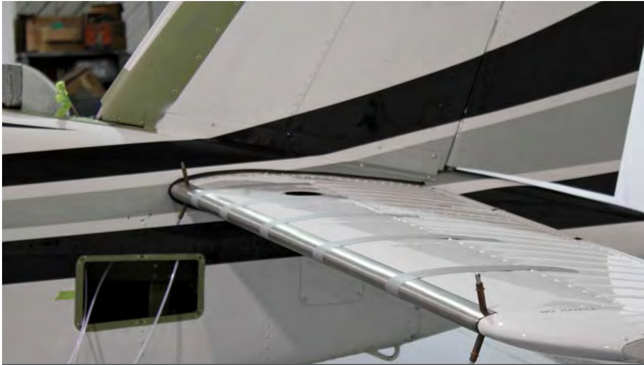
The rivets in the corners are sacrificial members, not intended to secure the panels to the aircraft.
