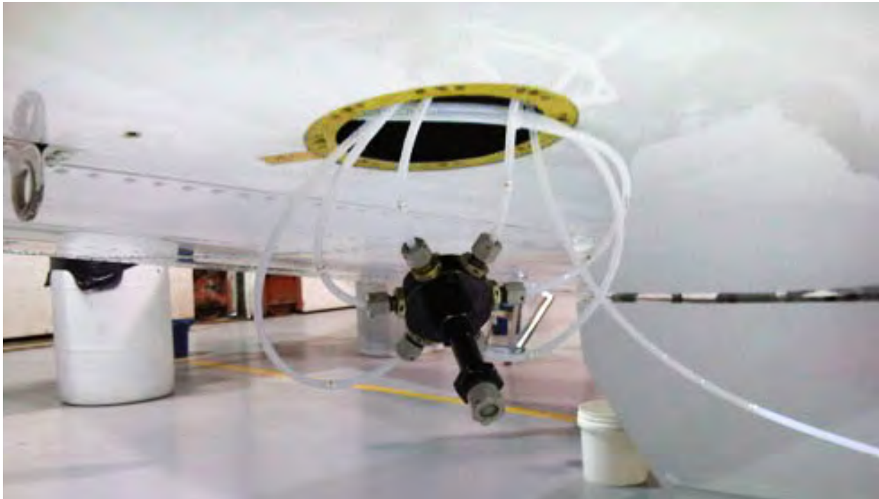
The fluid lines leading to the panels are disconnected from the aircraft's proportioning units and attached to test units.
