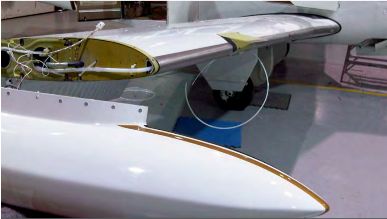
The tip tanks are replaced.
