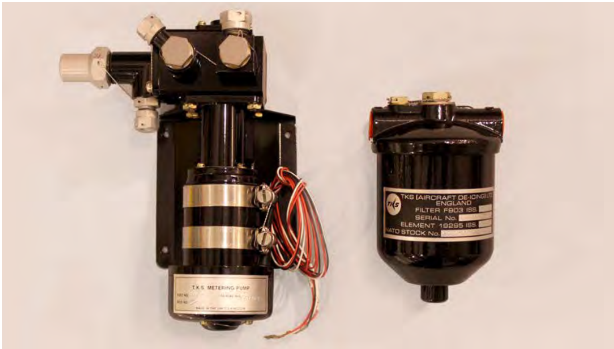
TKS Metering Pump and Filter.
