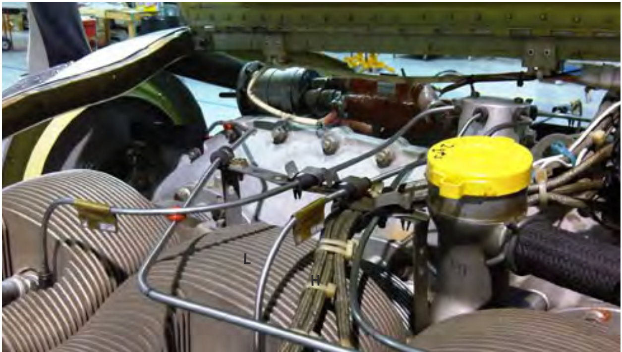
A stainless steel tube brings fluid over the engine.
