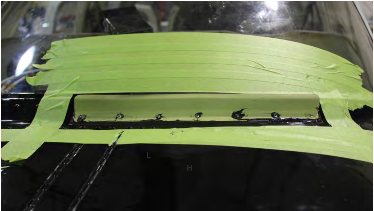
A deflector is bonded and riveted over the windshield spraybar.
