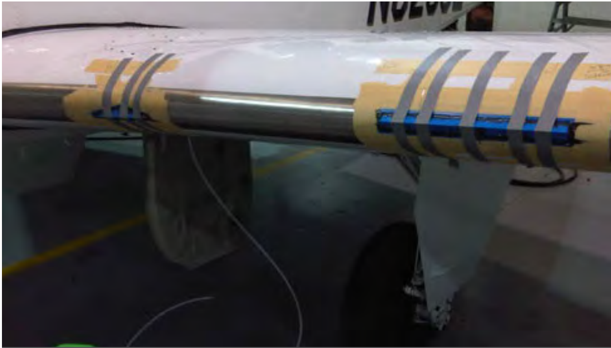
The stall strips are worked into the correct shape to fit flush against the panels, then bonded.
