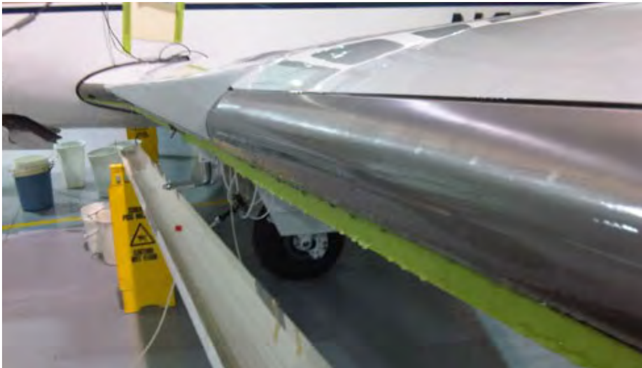
After the edge seal has cured, the TKS Ice Protection System undergoes testing. Panels are slowly brought to 70 psi in order to purge and check the flow. Under normal operation the panels will see 3-5 psi.
