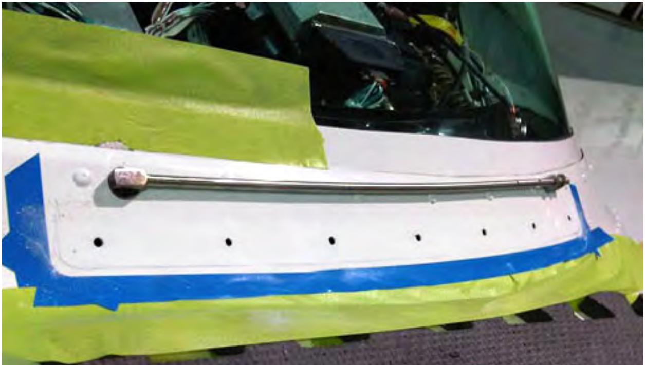
The windshield spraybar is installed under the left side screen.
