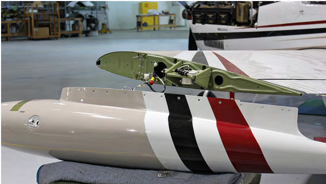
The r/s tip tank is pulled to allow routing for plumbing.
