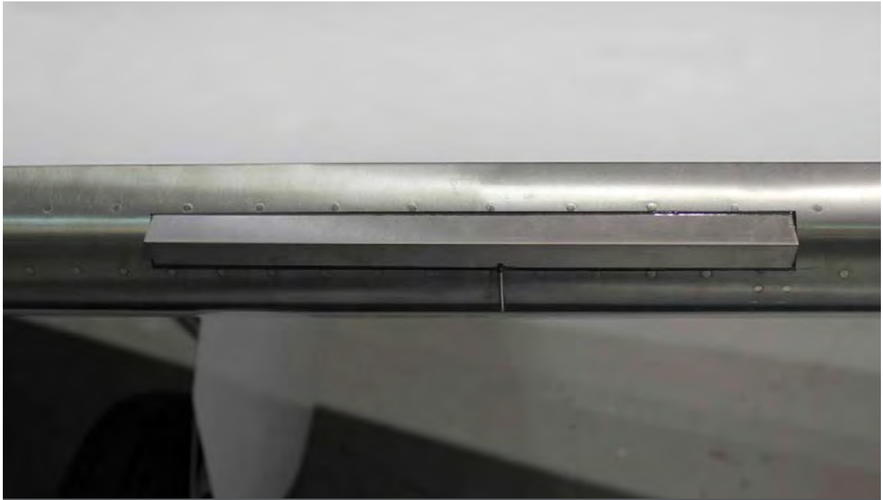
Stall strips for the leading edge are installed.
