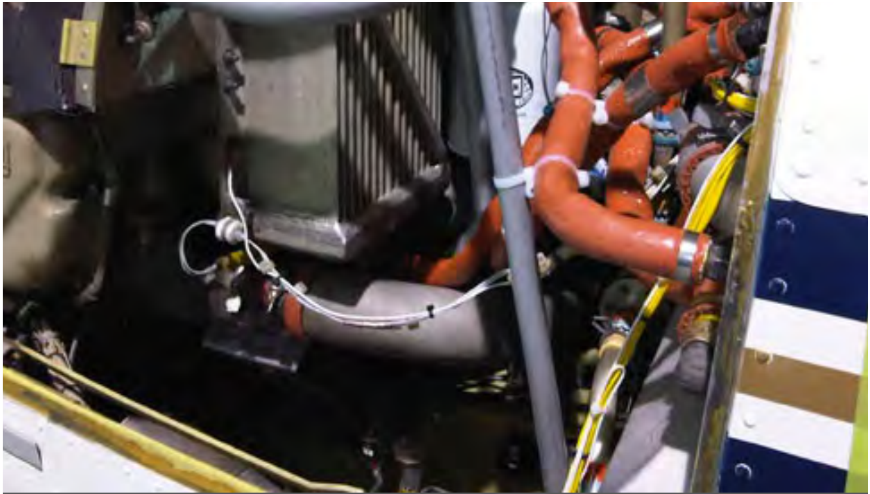
A firehouse is installed to bring the fluid to the prop.
