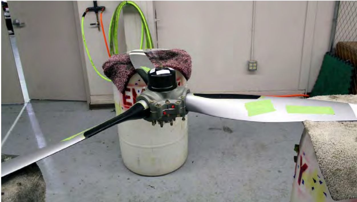
TKS boots are applied to the prop blades.
