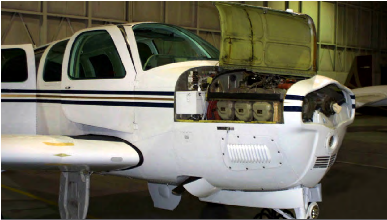
The prop is pulled and sent back to a dedicated workroom for slinger ring installation.
