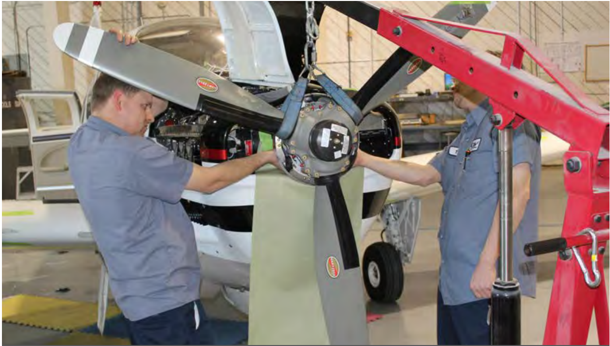
The prop is reinstalled and will be dynamically balanced toward the end of the third week.
