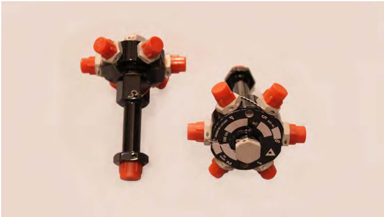
The six port proportioning unit is used in one of the wings. Its twin will be located in the adjacent wing. The three port proportioning unit is used in the tail to send fluid to each horizontal stabilizer and the vertical.
