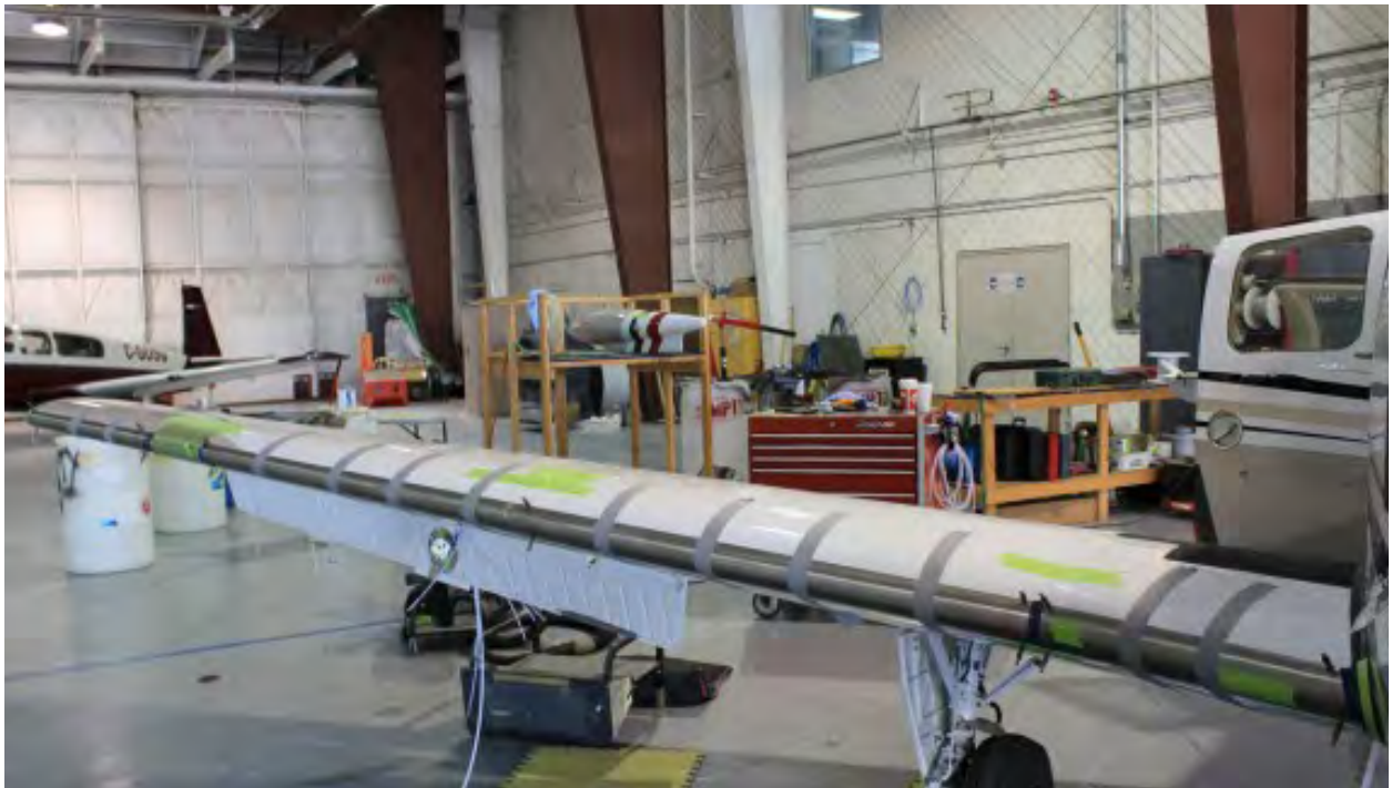
The initial fitting of the panels to the leading edge will be removed, trimmed and bonded.
