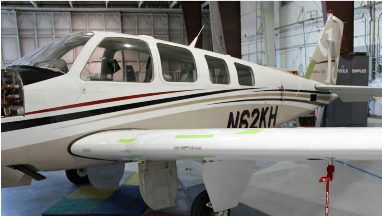
Stall strip locations are recorded and stall strips are removed. New, porous titanium strips will be installed over the TKS panels and will exude TKS fluid to help prevent ice accretion.
