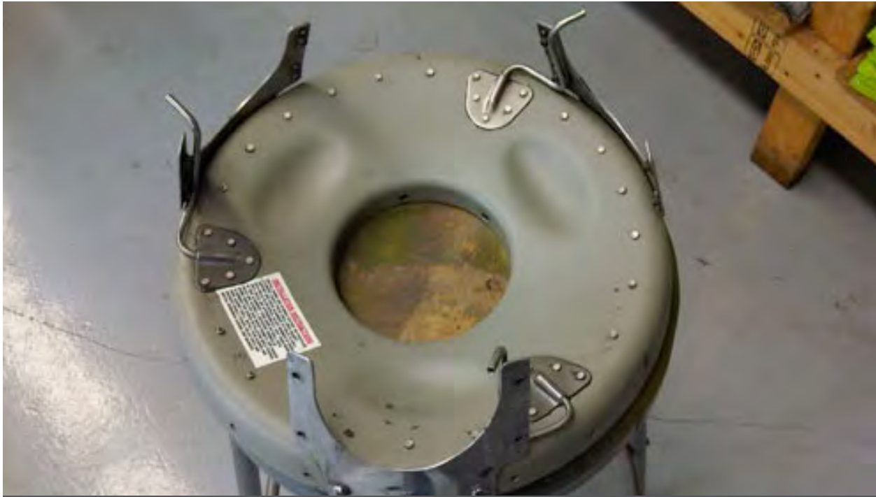
The slinger ring bonding agent has cured and the brackets, fluid scoops and feed tubes have been installed. The fluid is collected by the scoops inside the sling ring and passed through the feed tubes to the prop blades.
