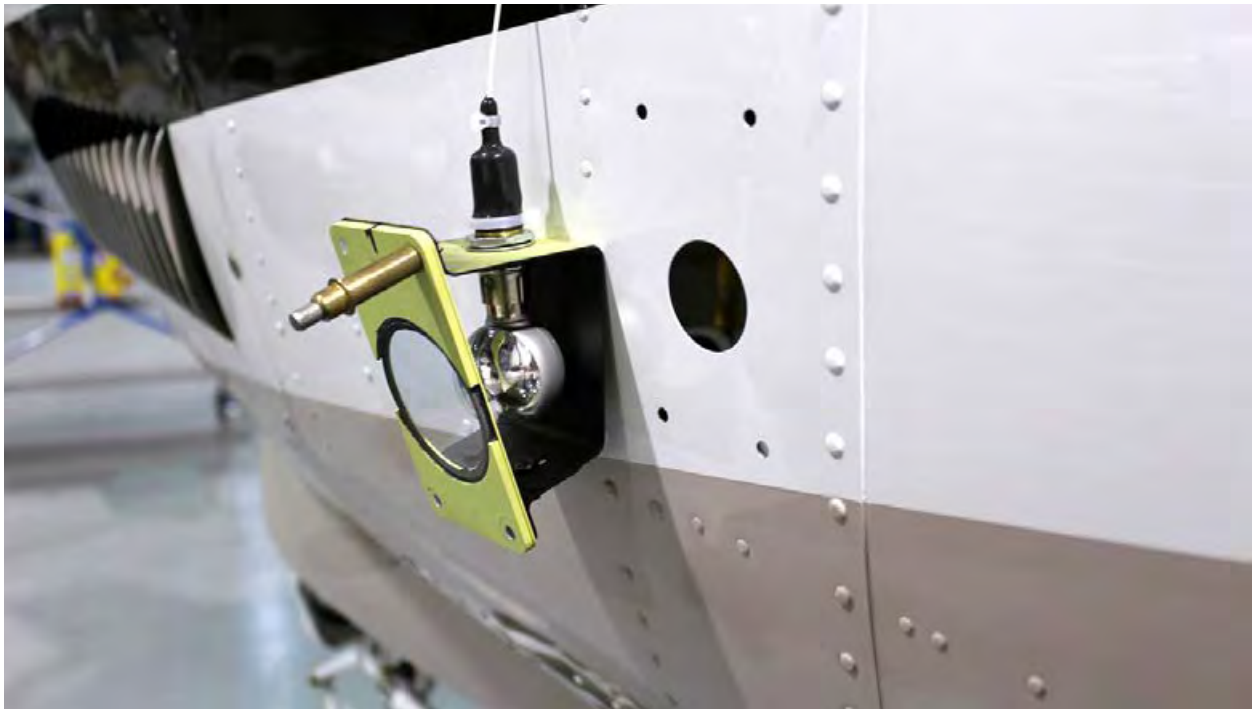
An ice light is installed in the left side cowling. The light will illuminate the left wing and is controlled by a switch on the TKS Ice Protection System Control Panel.
