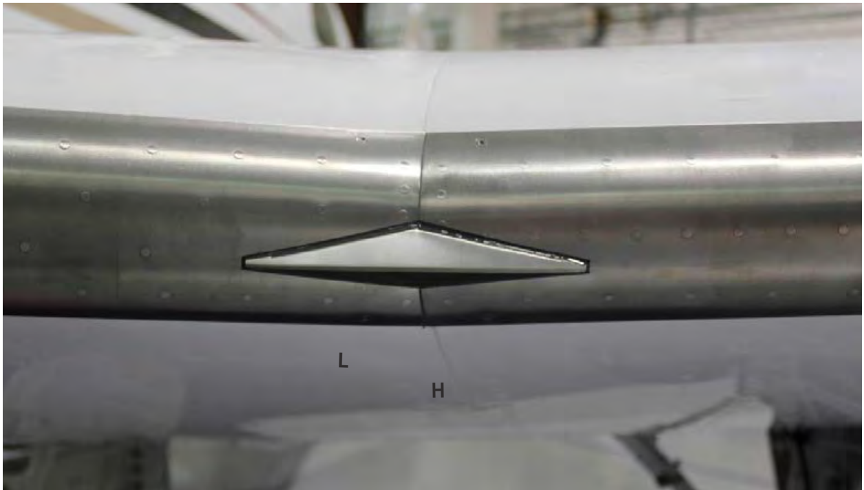
Stall strips for the wedges are also installed.
