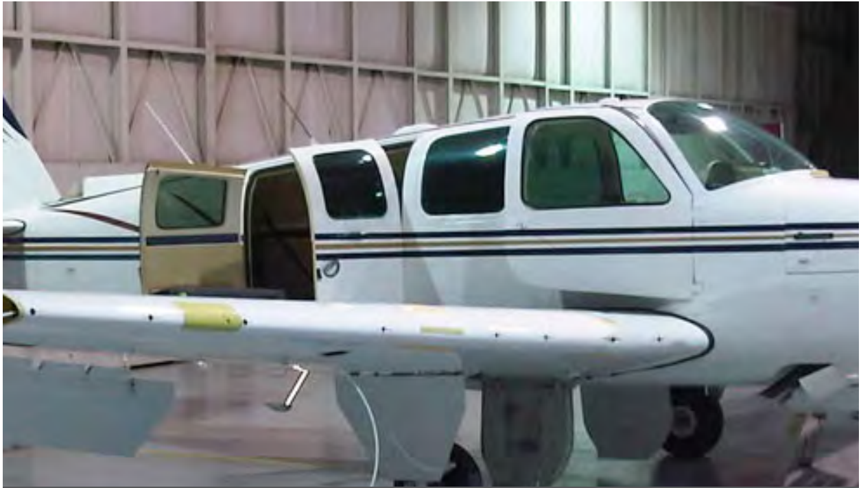
The TKS panels are pulled from the leading edge, then ground and formed to precisely fit.
