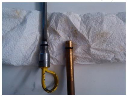
The air inlet fitting's outside diameter and o-ring groove dimensions are same as dip stick plug. It's easy to insert and remove with the engine hot, without getting oil on your clothes.
