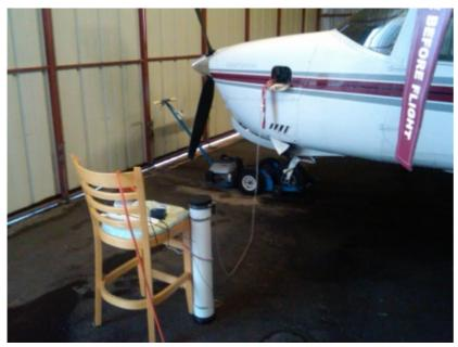
The dedydrator system connected to N4429L's engine, quietly doing its job. Dry air flows into the engine through the dipstick tube and exits mostly via the breather tube. Note the in-line gasoline filter in the line just before the dry air enters the engine. This prevents any dust or other particulate matter from entering the engine.
