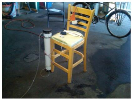
The structural supports (chair and bungee cord), the reactor column (4-in PVC pipe with rubber plumbing caps), the compressor (small aquarium pump), and digital controller (lamp timer).
