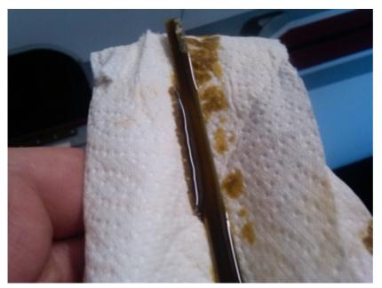
This oil has about 35 hours on it. It's difficult to see in this photo that the oil color is greenish-brown. Before using the dehydrator, the oil typically turned black by about 10 hours. Clearly the purging of moisture is having an effect.
