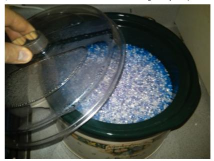
The desiccant after about one hour of regeneration. Note the condensation inside the lid showing that moisture is being driven off. The dye indicator is starting to turn blue around the edge where the heating element is.
