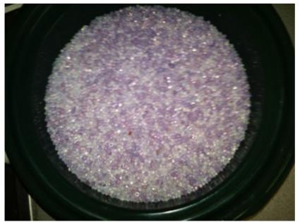
Saturated desiccant ready for regeneration, showing the mostly pink dye indicator with some flecks of light blue still showing. A charge of desiccant has been lasting about a month before regeneration is needed.
