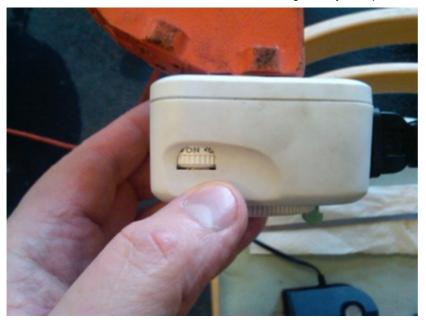
...turn the manual switch ON. The pump will now run for 24 hours, then 18 hours OFF, then 6 hours ON, repeating forever, or until you next stop it to go flying.
