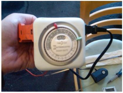
The timer ON and OFF trippers are 6 hours apart. To start the cycle, connect the hose to the hot engine, and rotate the timer wheel clockwise until the OFF tripper just turns the switch OFF. The time-of-day scale doesn't matter. Then...
