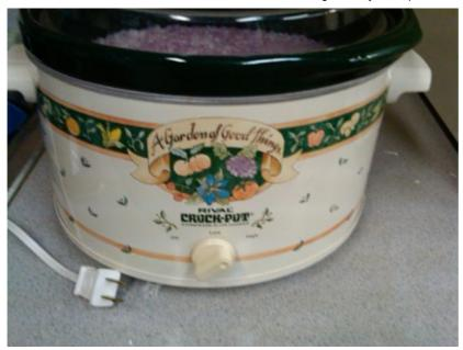
The desiccant reactivation reactor. On high setting the crock pot slowly heats up to about 220 deg F, which is ideal for regeneration. Higher temperature won't hurt the desiccant itself, but will ruin the blue-pink dye indicator. Also, rapid temperature changes can cause the desiccant to fracture and turn into dust. This doesn't happen in the crock pot as the heating is gradual, but be careful if you decide to use an oven or other method for regeneration.
