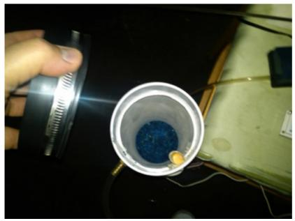
Removing the top rubber cap shows the inside of the desiccant column. The column is about half full of silica gel. Air enters at the bottom and flows upwards through the desiccant, so the desiccant at the bottom becomes saturated first. The blue color at the top indicates the desiccant still has capacity to absorb moisture.
