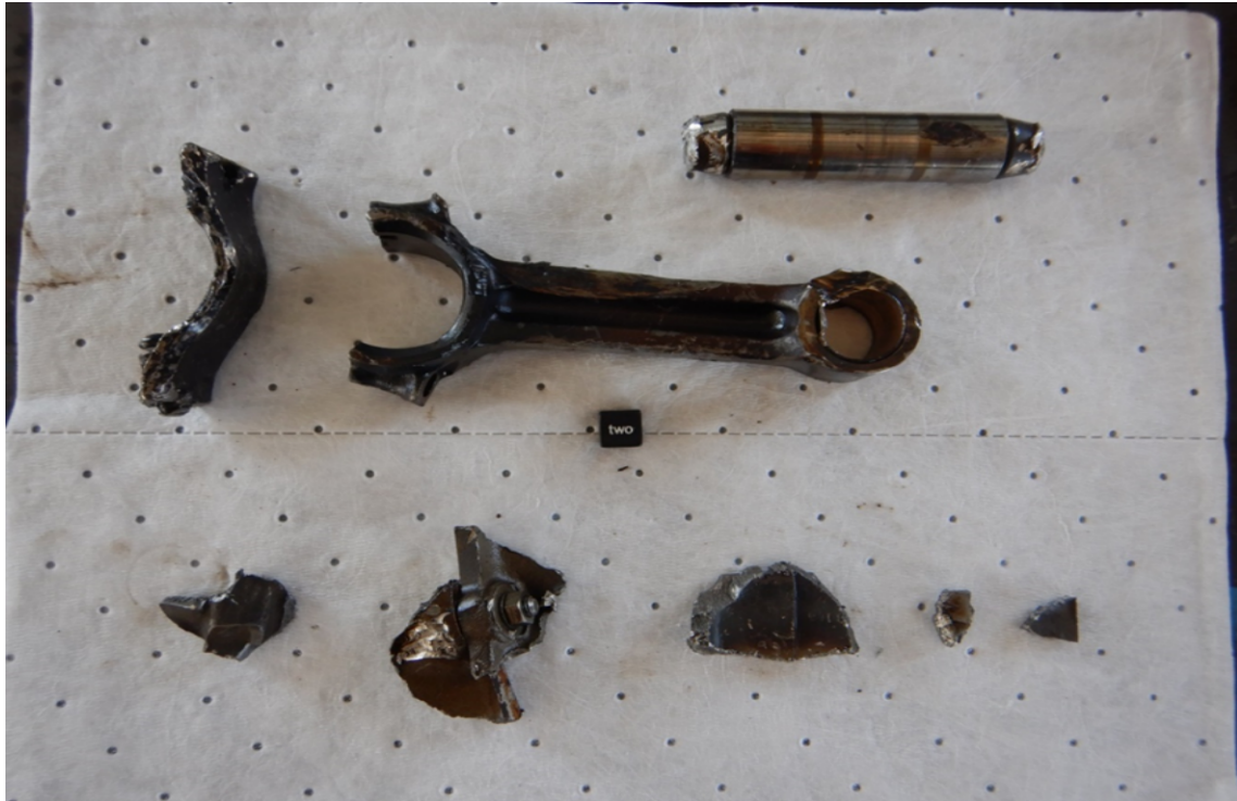
Figure 2. No. 2 connecting rod, piston, crankcase pieces, and piston material.
