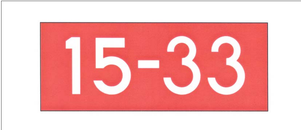
FIG 2-3-24 Runway Holding Position Sign
