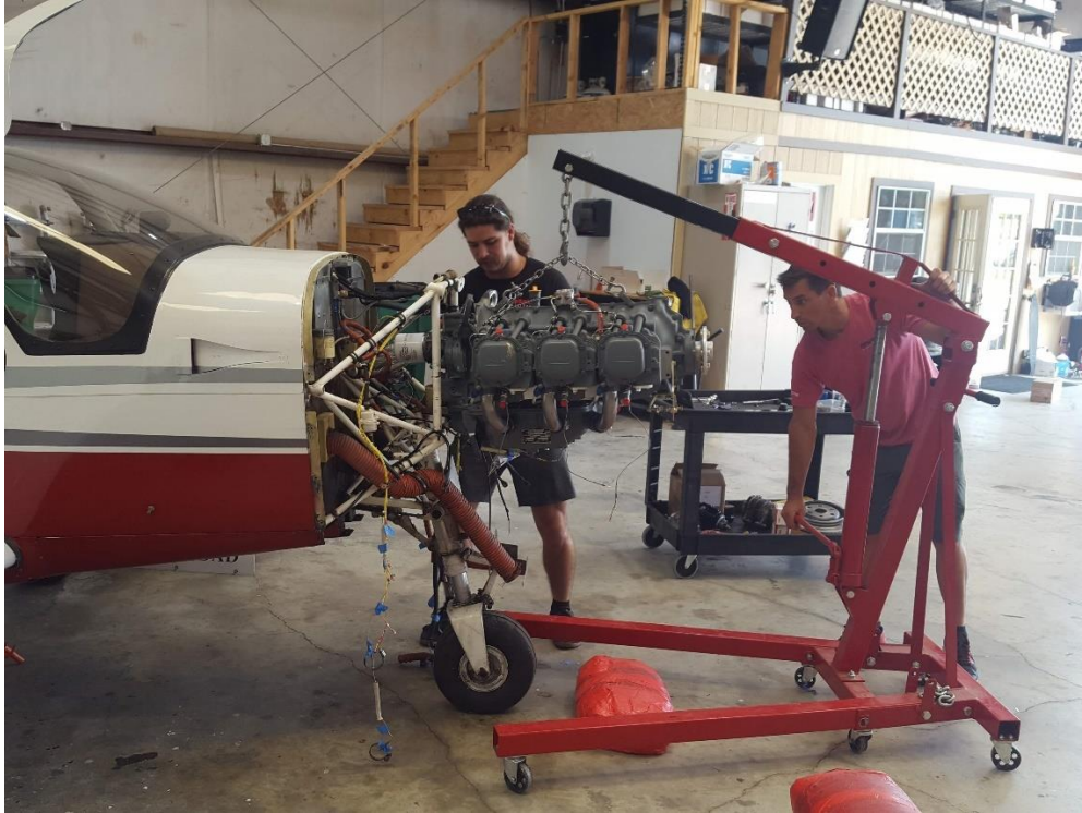
Figure 32: Engine attachment begins.
