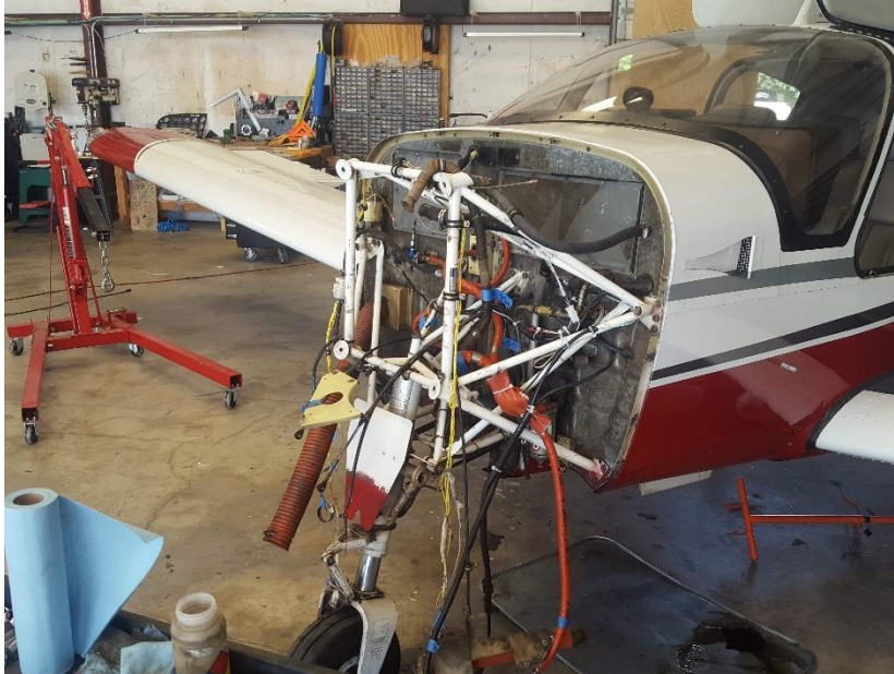
Figure 29: Engine removed for airframe.
