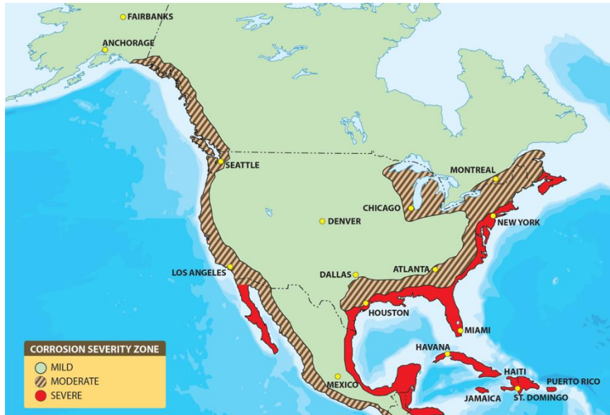
Figure 8: North America corrosion severity chart. From www.aircraftsystemstech.com/2019/02/factors-affecting-corrosion-in-aircraft.html
