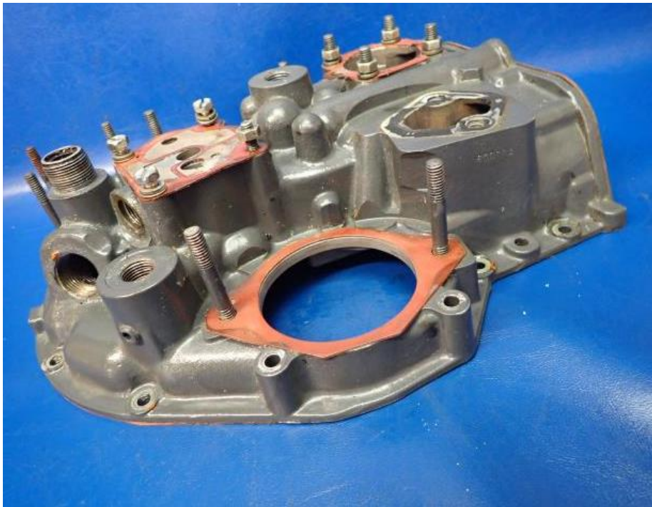
Figure 17: The accessory cases are not just two dimensional, they are three and can be seen better here. This case is for -C4D5 or -C4B5 engine.
