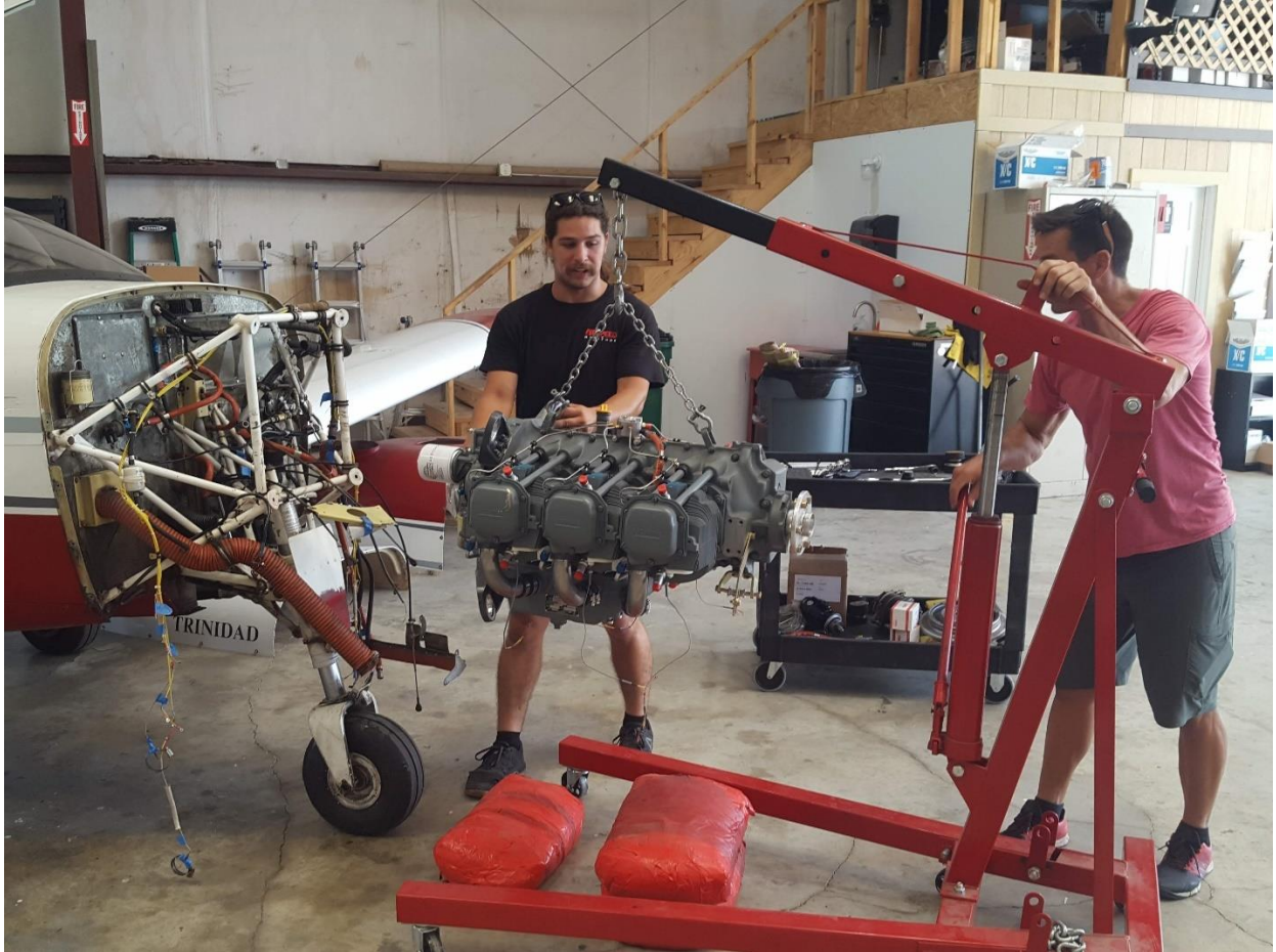
Figure 31: New engine moved into position.
