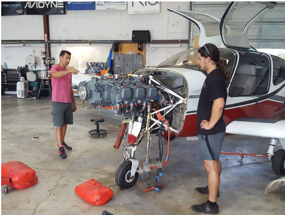
Figure 33: Engine attached to airframe and hoist removed. Ready for the accessories and other parts to be attached. Three people were performed the install of the engine. Anthony Arispe (left) owner of Airspeed and Altitude with two of his employees Connor (right) and Mikey (not shown).
