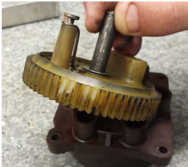
Figure 6 - SDR 510019629 Broken teeth
