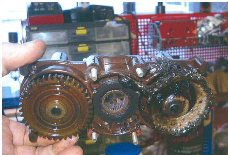
Figure 23 - Missing bearing retainer plate screws
