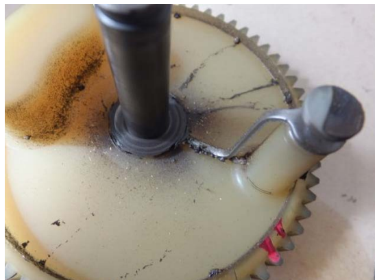
Figure 4 - Arcing damage on distributor gear wheel
