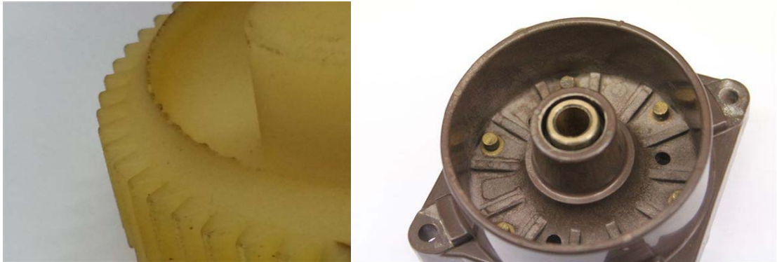
Figure 10 - Eroded gear and block
