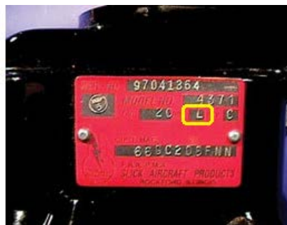
Figure 2 - Data plate showing typical code for direction of magneto rotation
