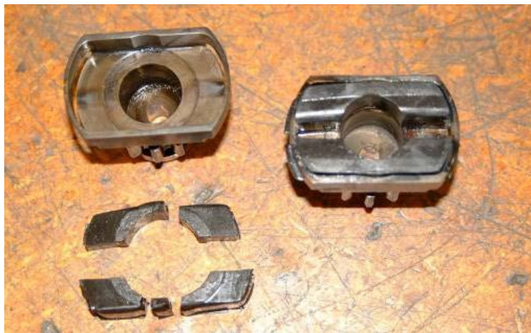
Figure 25 - Failed magneto drive rubbers
