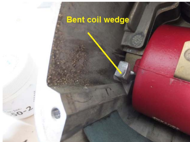
Figure 21 – Bent coil wedge
