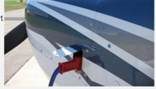
button. When connected to ground power, a cowl mounted piezo-electric switch activates the system without ever opening the cabin door. **Your lineman can do it for you.**
