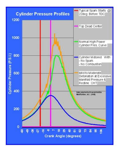
The vertical red line is the spark, the pink is TDC. The blue curve is the pressure you might see with "no fire," the green is the pressure pulse with normal high power, and the orange is detonation, about which, more later.
