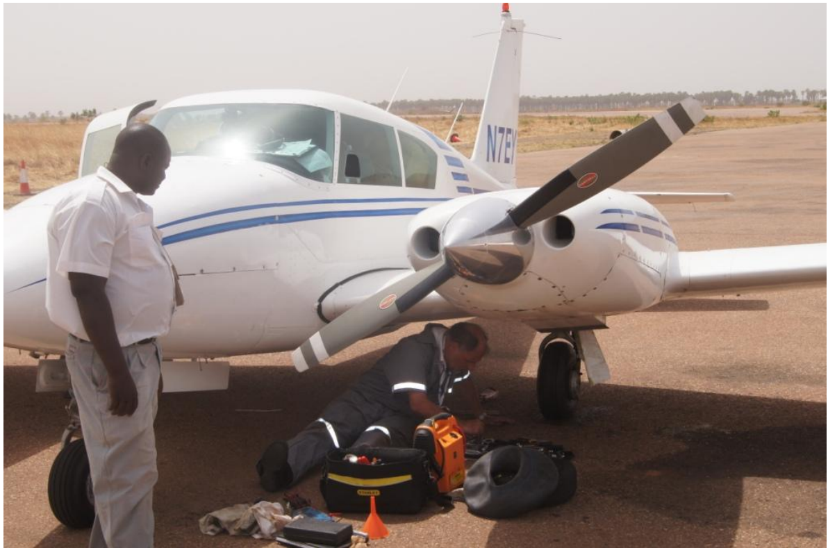
Final checks to the replacement tyre and wheel
